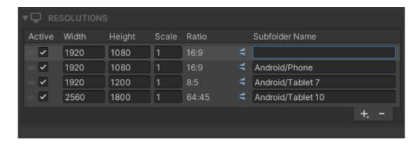
You can remove any resolution form the list by highlighting it and pressing the - button
