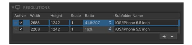
First click the + button located at the bottom of the Resolutions list.
